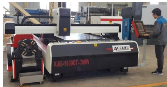
Figure 1: ACCURL laser tube cutting machine in operation
